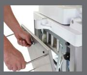
Maintenance side access with the unlocking system **Quick Access** that makes daily cleaning inside the machine much easier.
