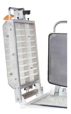
The plastic material of the grids guarantees a softer cutting that allows the dough pieces to be resolded at the extremities after the division. Gently shaped, the dough will give breads with rounder extremities and a score opened nicely. The signature of each baker is preserved at each batch!
